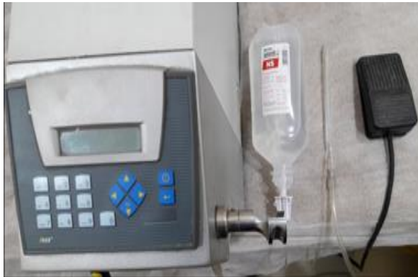
Fig. 1: Control panel with source of pressurized oxygen, tubing line accessories, a sterile disposable hand piece, sterile water/saline bag, footswitch
